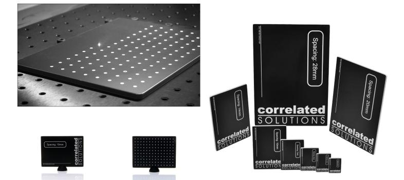
The new calibration targets are fabricated from an aluminum sandwich material with a polymer core providing ultimate rigidity. The aluminum faces are anodized for contrast and increased durability. The calibration targets are also specially coded, enabling the analysis software to automatically detect the spacing of each target, increasing the overall robustness and ease of use of the VIC-3D system.
