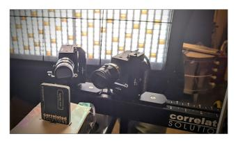
Correlated Solutions is also now offering low-resolution calibration targets for cameras with less than one megapixel in total resolution. This is common with ultra highspeed cameras such as the Shimadzu HPV-X2. The targets have fewer and larger markers, which allows VIC-3D's algorithms to locate the centroids with more accuracy and consistency, improving the overall stereocalibration and analysis results.
