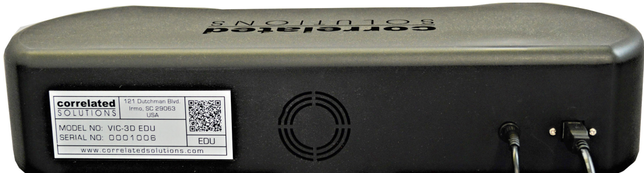
Figure 3: Photograph of back panel for VIC-EDU measurement head. Rectangular USB cable is for the cameras. Round cable is the power supply connection
