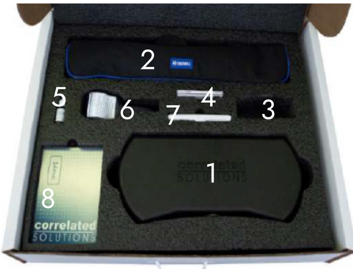
Figure 1: Top view of contents in VIC-EDU vibration-protected case
